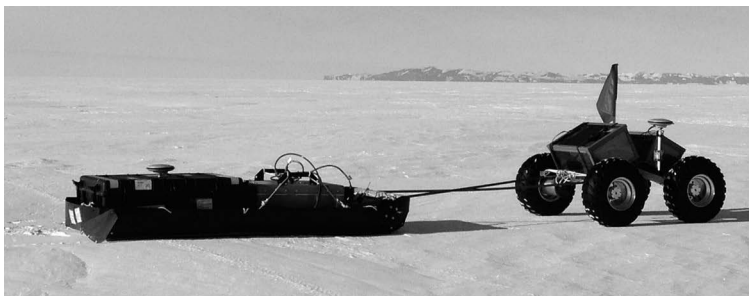
FIGURE 12.2 Yeti crevasse sensing autonomous. (Courtesy of Laura E. Ray, professor of engineering at Dartmouth College and Yeti project leader.)
